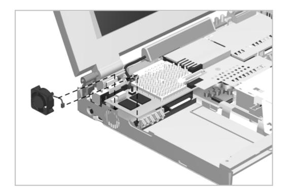
Figure 5-48. Removing the Fan
